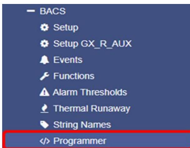
Regular BACS Operation must be interrupted during programming of modules. Enable this page to halt bus polling and disable this page again when done, to restart BACS Operation.
