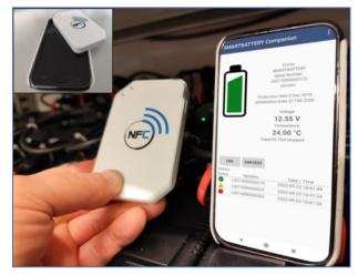
The SMARTLOGGER / SMARTBATTERY is the first battery monitoring device on the market that can do both: Data evaluation and long-term recording in accordance with the European Battery Act 2024.
