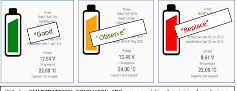
With the SMARTBATTERY COMPANION APP, you can define threshold values that are individually adapted to the location and contractual conditions, which can be used to immediately determine whether potential operation outside of the specifications has occurred during regular on-site maintenance.
