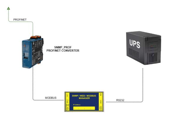
The SNMP\_PROF **PROFINET converter** is a versatile and powerful device specifically designed for the seamless integration of Modbus-based devices into PROFINET networks.
