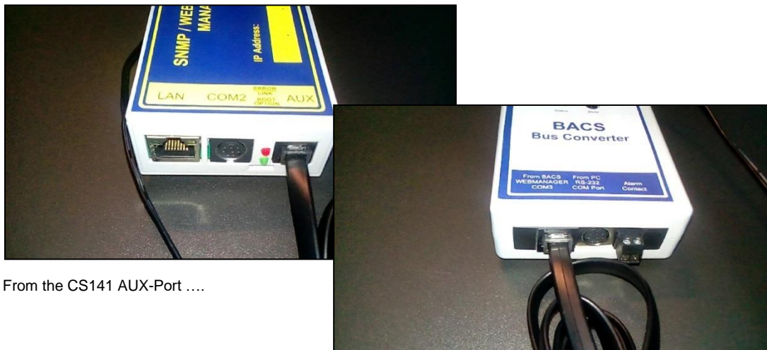
... to the COM 3 port of the BACS-Bus Converter
