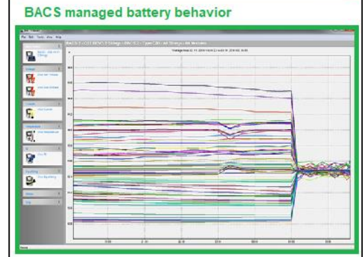
BACS® VIEWER SCREENSHOT As seen by BACS®, the same 5-year-old system as shown in the previous graphic, this time, after the application of the genuine Equalization (Balancing) process. Within a few hours, this process brings the variance in float voltage to within 1/100 th of a volt of the level recommended by the manufacturer.
