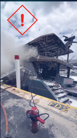
Total loss of the yacht 'Flagship' following BMS failure (NTSB MIR-25/31)
