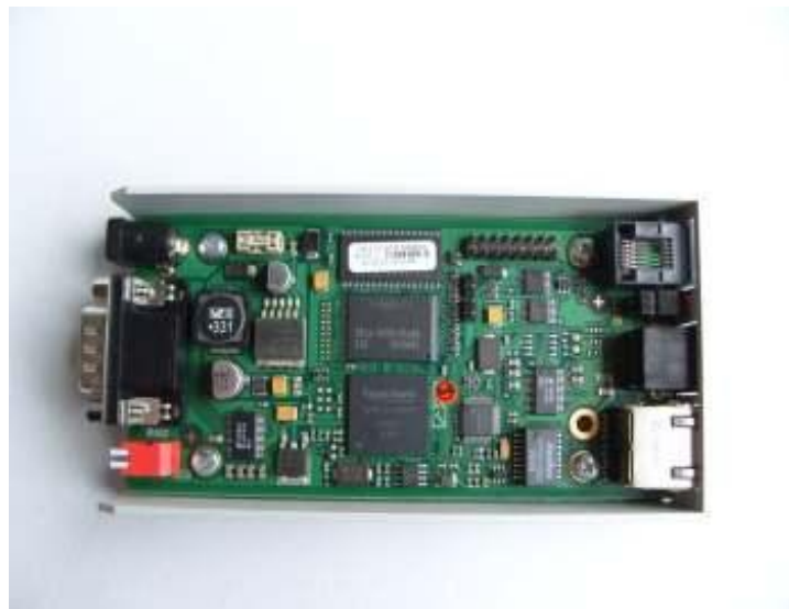
BACS II Webmanager Budget I, external aluminum chassis, open
