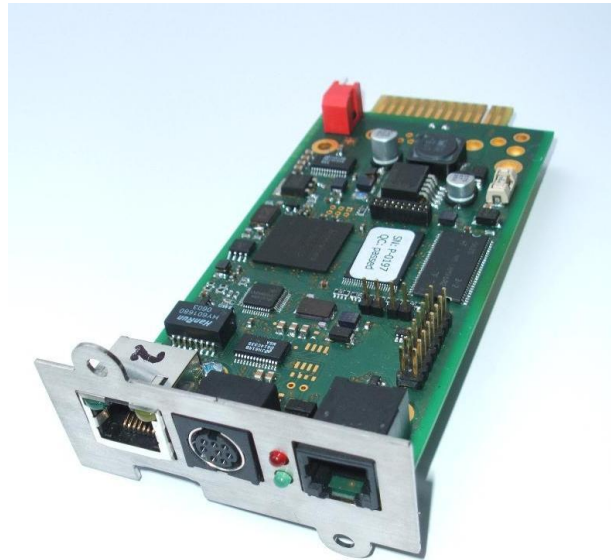
BACS WEBMANAGER BUDGET 2 - (HW131), SC slot card version, front side
